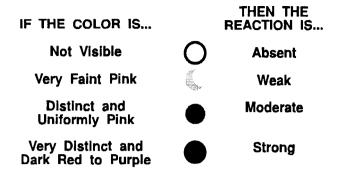
Reactions may appear in any shape (i.e., rings, crescents, dots) and should be interpreted for color intensity only. Any colored shape in the test spot of greater intensity than the negative control spot, should be interpreted as a positive result.
